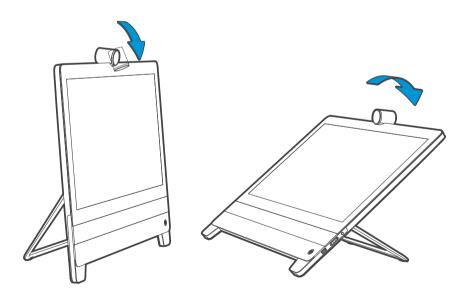
You can tilt the camera to adjust the camera angle and to activate the document camera feature.
