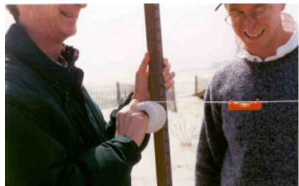
Figure 1-5: The line level is “level” and the string is used to determine the elevation reading on the long rod.
