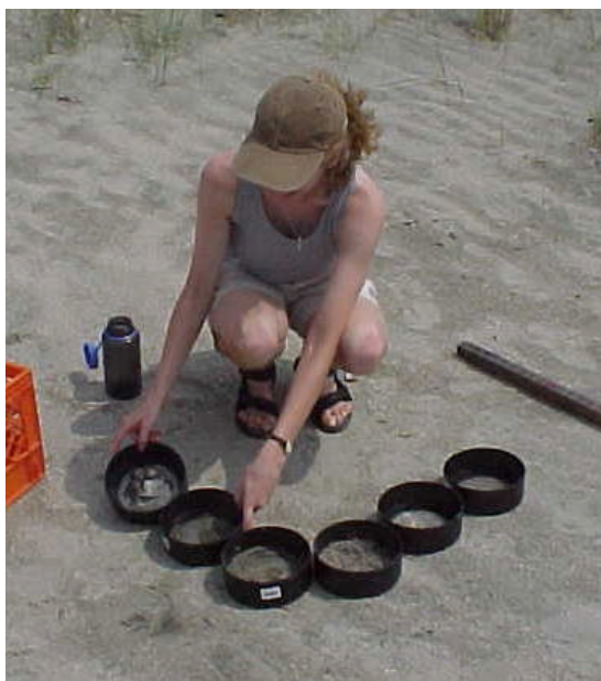
Figure 2: Sediment has been sorted and distributed among the six sieves. (Photo courtesy of Angela Mills)
